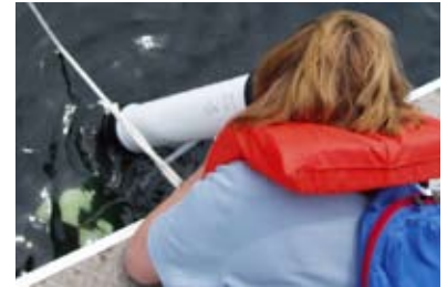
Measuring water quality with a Secchi disk helps us to understand the influence of development on our lakes.
